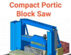
DOUBLE BRIDGE COMPACT CUTTING CAR MODEL defined by max. cut - 58in / 1,47 mt; Min.periph.speed:20 mts/sec
