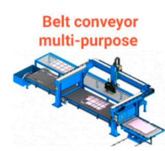
HERCULES SERIES GAMA 300 & 500 MODEL defined by max. cut - 14.1/2 in / 37 cm; Bridge lenght 236 in / 6 mt
