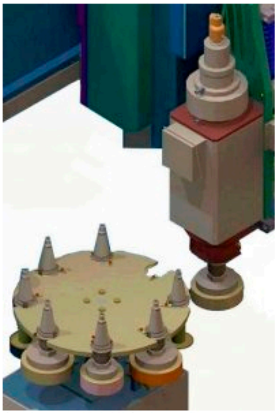
Carrossel Tool Change Provide the work with multi-tools, best to use on spindle
